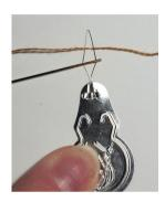
Step 2: Pass the thread through the wire, above the needle.
