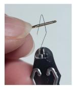
Step 1: Pass the wire through the eye of the needle.
